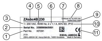
Name plate using the ZAsbc4B 230 as an example
