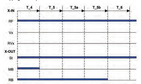
T\_4 Hold speed 0T\_5 Wait until the brake is closed
