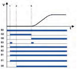
Quick start with DCP actuation B0 Converter enable
