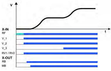
Starting with acceleration from V\_1 to V\_2
