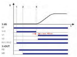
Quickstart with standard actuation RF Controller enable v=0 Hold speed 0 V1 Positioning speed V3 travel speed RV1 / RV2 Direction RB Controller ready MB\_Brake Mechanical brake
