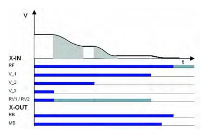
Normal stop with distance-dependent deceleration and deceleration from V\_3 to V\_2.
