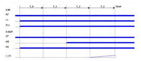
T\_0 Time until motor contactors have been opened
