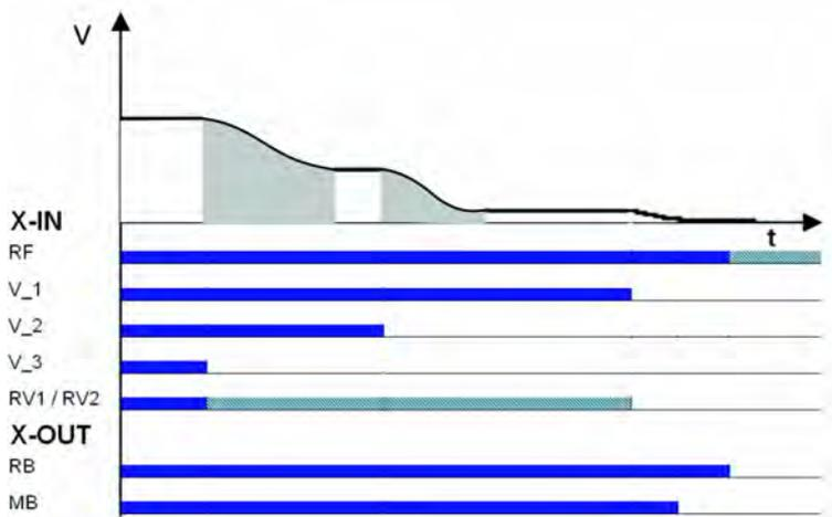
Normal stop with distance-dependent deceleration and deceleration from *V\_3* to *V\_2*.
