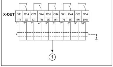
Connection of the digital outputs X-OUT
