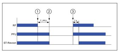
Function of stand-by mode of power recuperation unit type REVCON RLD 1 End of travel
