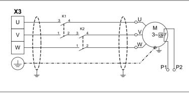
Asynchronous motor connection
