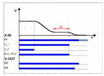
Deceleration with non-optimized crawl path *RF Controller enable* V\_1 Positioning speed
