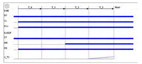
T\_0 Time until motor contactors have been opened
