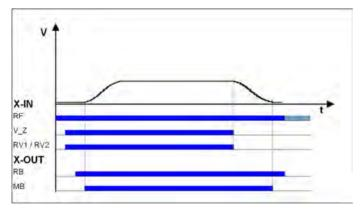
Readjustment speed *RF* Controller enable *V\_Z* Readjustment speed *RB* Controller ready *MB\_Brake* Mechanical brake
