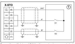
Connection with internal 24 V voltage using two separate jacketed cables
