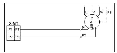
Temperature monitoring connection () terminal designation of connector
