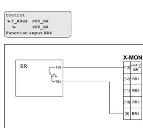
Connection brake resistor
