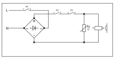
Brake control principle circuit diagram
