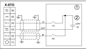
Connection with external 24 V voltage using two separate
