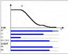
Deceleration ramp *RF* Controller enable *V\_1* Positioning speed *V\_3* High travelling speed *RV1 / RV2* Direction default *RB* Controller ready *MB\_Brake* Mechanical brake
