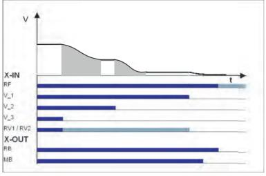
Normal stop with distance-dependent deceleration and deceleration from V\_3 to V\_2.
