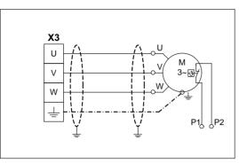
Connection asynchronous motor / synchronous motor
