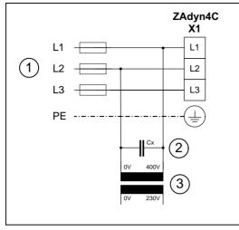
Control transformer in the mains feed line
