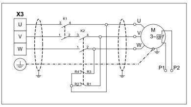
Synchronous motor connection
