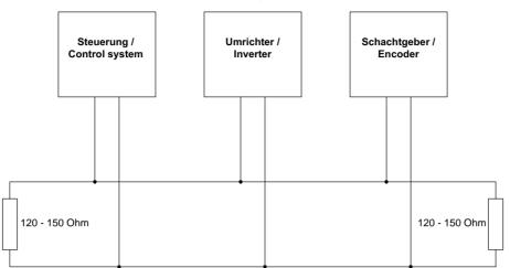
Exemplary assembly of a bus-system with CANopen
