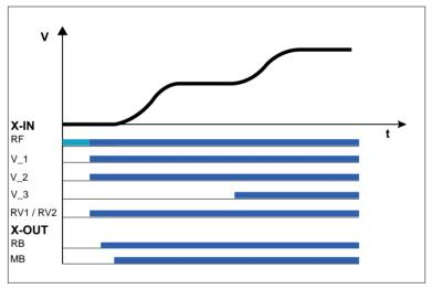
Starting with acceleration from V\_1 to V\_2
