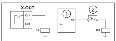
Actuating the brakes via the frequency inverter and control
