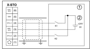
Connection with external 24 V voltage and protected routing jacketed cables
