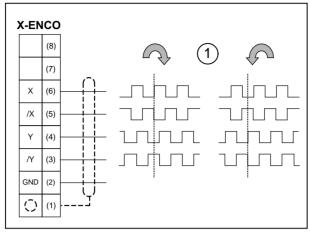
Connection of rotary encoder simulation
