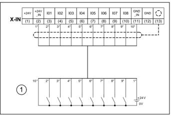
Connecting digital inputs to external power supply with inverted logic
