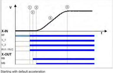
Starting with default acceleration *RF* Controller enable *V*\_1 Positioning speed *V*\_3 High travelling speed
