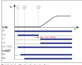
Quickstart with standard actuationRFController enablev=0Hold speed 0V1Positioning speedV3SpeedRV1 / RV2Direction defaultRBController readyMB\_BrakeMechanical brake
