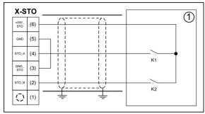
Connection with internal 24 V voltage and protected routing 1 Brake control Brake control
