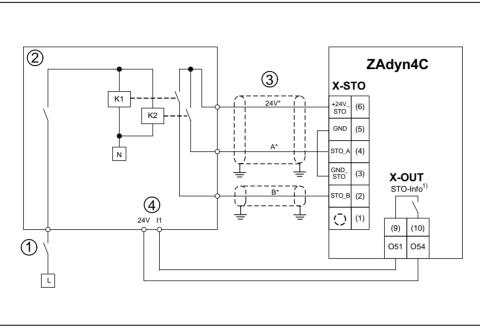
Principle circuit diagram "Safe Torque Off (STO)" function
