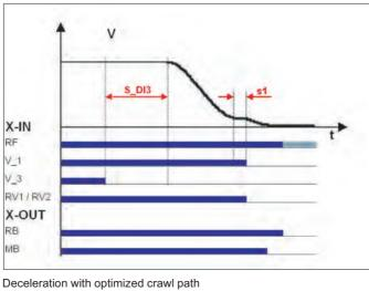
RF Controller enable V\_1 Positioning speed V\_3 High travelling speed
