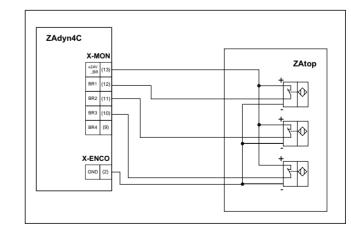
Connection of brake release monitor with initiators
